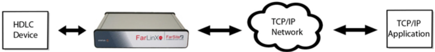
Diagram illustrates an application running on a TCP/IP network connecting to a device with an HDLC connection. The FarLinX Connect Mini providing the conversion between TCP and HDLC
